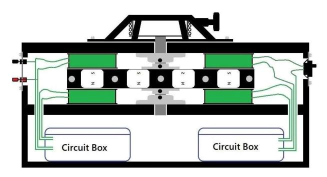
I can't give you exact measurements for the side and bottom of the box. You'll have to take measurements off the Rotor Assembly. What you're going to do is make three sides and a bottom to be attached to the Rotor
