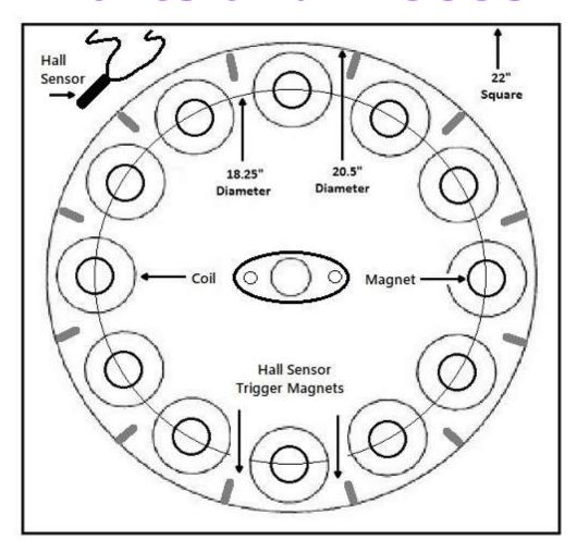
You need 3 pieces of 3/4" plywood 22" square. find center and mark a 18.25" circle on both and one 20.5" plywood Disk the same thickness as your magnets.
