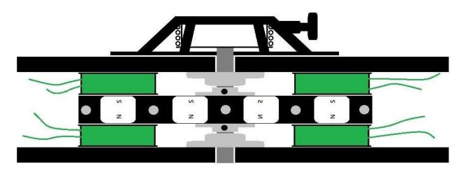
If you've been making the parts as you go through the manual you should now have the Magnets installed in the Rotor the Coils made and Glued to the square panels and the Rotor Shaft made.
